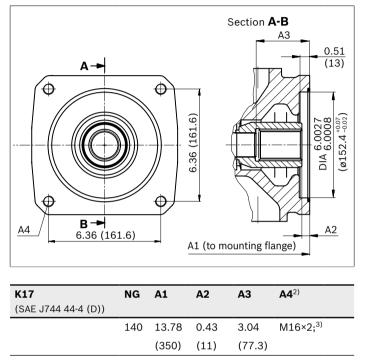
According to ANSI B92.1a, 30° pressure angle, flat root, side fit, tolerance class 5 3) Continuous
