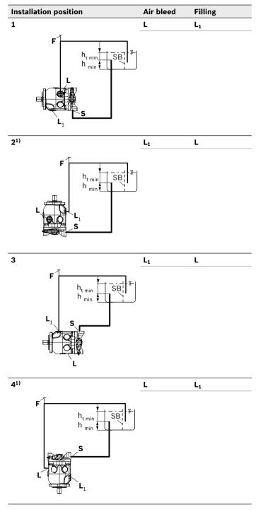
Because complete air bleeding and filling are not possible in this position, the pump should be air bled and filled in a horizontal position before installation.
