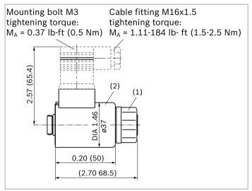
The seal ring in the cable fitting is suitable for lines of diameter 0.18 in to 0.39 in (4.5 mm to 10 mm). The mating connector is not included in the scope of delivery. This can be supplied by ATUS on request.
