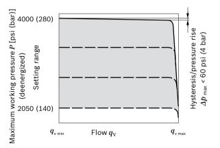
Characteristic curve valid at  $n_1 = 1500$  rpm and  $\theta_{fluid} = 122$  °F (50 °C).
