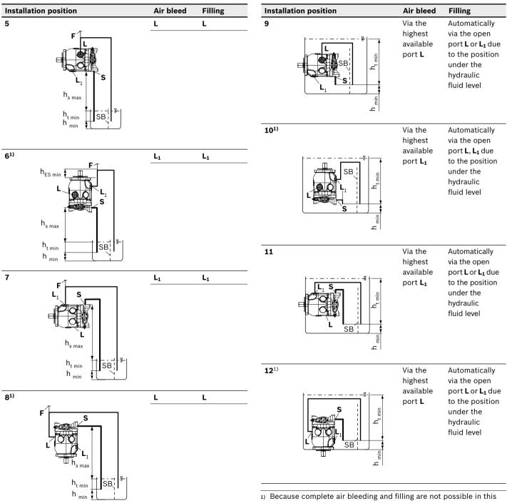
position, the pump should be air bled and filled in a horizontal position before installation.
