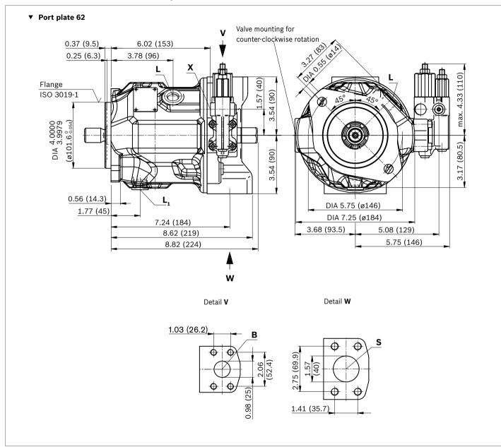
DFR/DFR1 - Pressure flow controller, hydraulic, clockwise rotation
