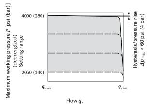
Characteristic curve valid at  $n_1 = 1500$  rpm and  $\theta_{fluid} = 122$  °F (50 °C).
