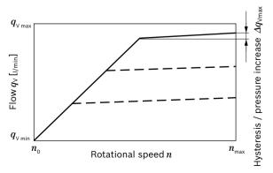
Characteristic curve valid at  $n_1 = 1500$  rpm and  $\theta_{fluid} = 122$  °F (50 °C).
