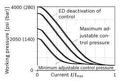
Hysteresis static current-pressure characteristic curve < 45 psi (3 bar).</li>
