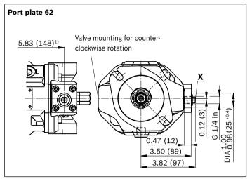
▼ DRG – Pressure controller, remote controlled
